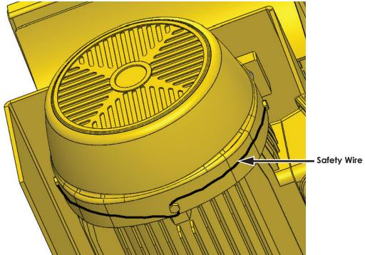
Figure 1: Safety wiring for M8 long screws
