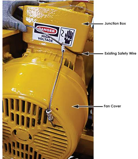
Figure 3: Other end of safety wiring secured to existing loop
