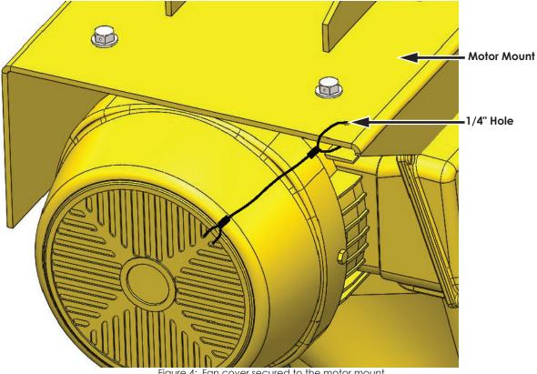
Figure 4: Fan cover secured to the motor mount
