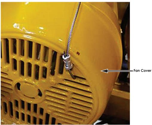
Figure 2: Safety wiring through the mesh in fan cover
