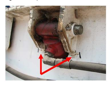
Figure 2 - Example of cracks on the "Driller Side"
