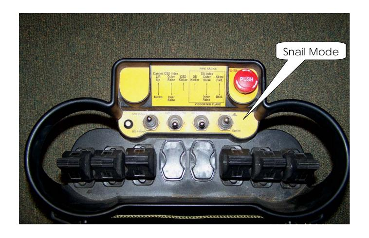
4. Once the carrier is firmly against the safety bar, continue to hold the carrier joystick in the down position and slacken the carrier cables until they can be unpinned from the carrier cable block without excess difficulty (in the event the pins cannot be removed without disconnecting the cables from the block).
