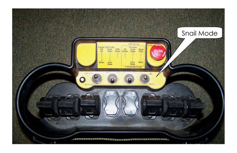
4. Once the carrier is firmly against the safety bar, continue to hold the carrier joystick in the down position and slacken the carrier cables until they can be unpinned from the carrier cable block without excess difficulty.
